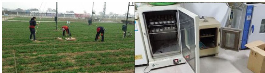
Fig. 7.8 Soil sampling and oven-drying weighing
