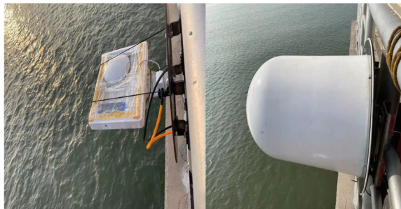
Fig. 6.30 Test scenario for measuring sea surface height with a smartphone
