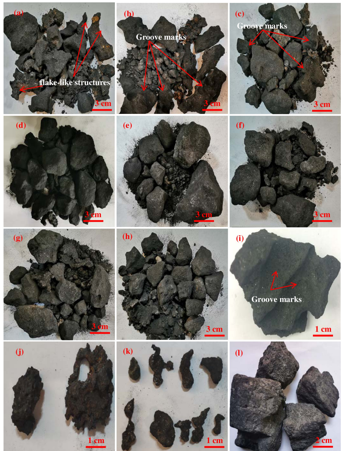
Fig 3. Macromorphologies of the coke in the hearth. (a) Sample ① at 0 m horizontal and 1 m vertical; (b) Sample ② at 2 m horizontal and 1 m vertical; (c) Sample ③ at 4 m horizontal and 1 m vertical; (d) Sample ④ at 6 m horizontal and 1 m vertical; (e) Sample ⑤ at 7.5 m horizontal and 1 m vertical; (f) Sample ⑥ at 7.5 m horizontal and 2.4 m vertical; (g) Sample ⑦ at 7.5 m horizontal and 3.8 m vertical; (h) Sample ⑧ at 7.5 m horizontal and 5.2 m vertical; (i) coke eroded by liquid metal at 0–2 m horizontal and 1 m vertical; (j) slag and iron at 0–4 m horizontal and 1 m vertical; (k) slag and iron at 6–7.5 m horizontal and 1 m vertical; and (l) original coke.
