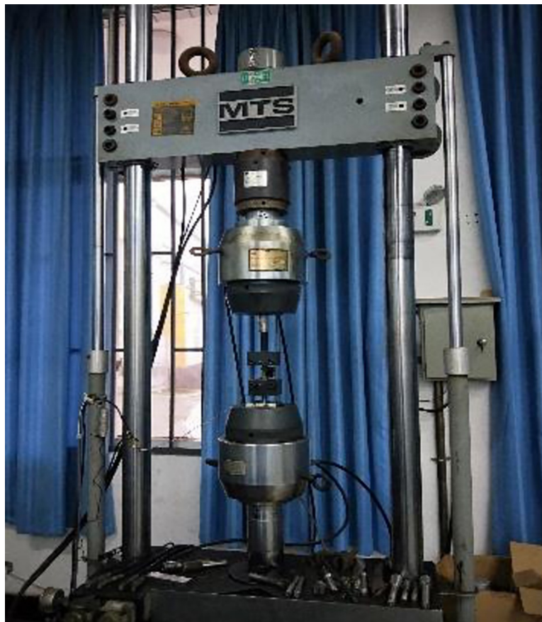
Fig 5. MTS hydraulic universal testing machine.
