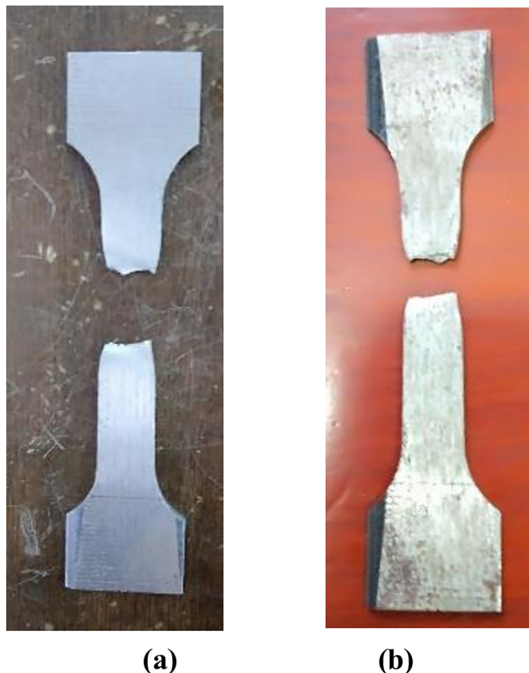
Fig 11. Fracture morphology of sample after tensile test. (a) Before corrosion and (b) After corrosion.
