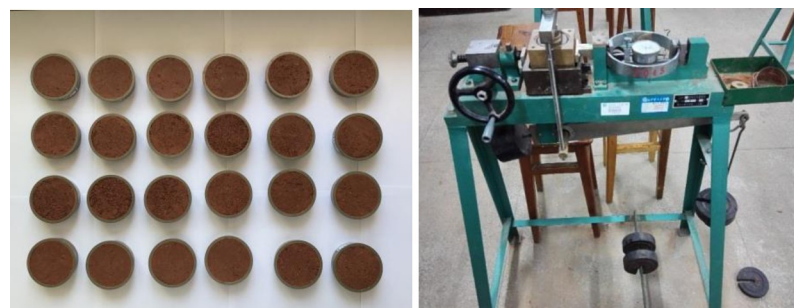
Fig 4. Planted soil composite with ring knife sampling and direct shear apparatus.
