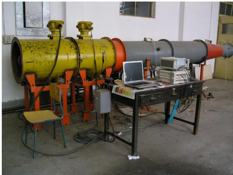
Fig 1. KDF-5 low noise contra-rotating fan and main experimental facilities.
