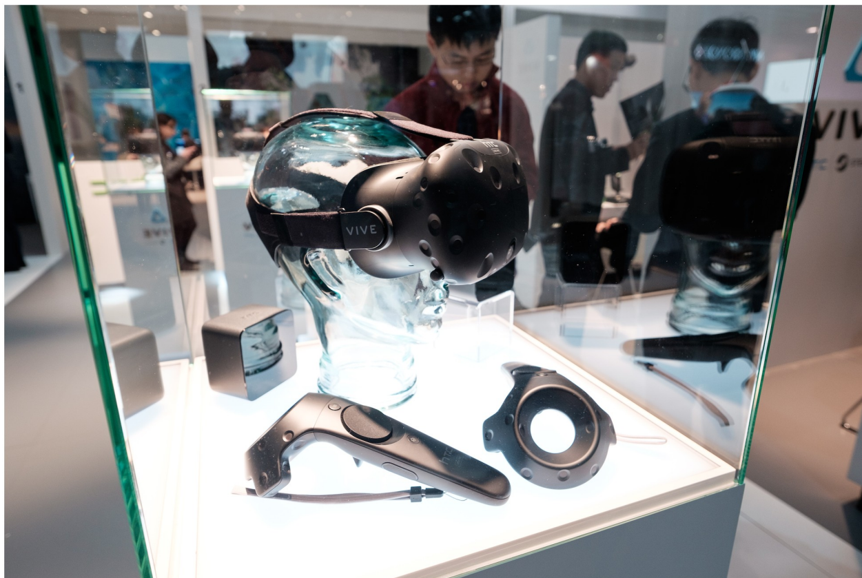
Fig 1. HTC Vive Virtual Reality system with a head-mounted display (top center), tracking device (left) and input devices (bottom left and right).
