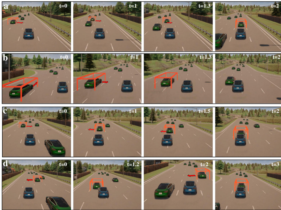
Fig. 8 Adversarial examples generated in NADE. a The autonomous vehicle (AV, blue vehicle) was on high speed and had a rear-end collision with the cut-in principal other vehicle (POV, green vehicle with orange rectangle) after two front-left POVs sequentially changed their lanes towards the AV. b The AV made a left lane change and collided with the POV due to a lane conflict (the POV accelerated first and then made a right lane change, simultaneously with the AV). c The AV turned left to avoid the collision to the cut-in POV but failed as the cut-in POV switched back to the left lane simultaneously with the AV. d The AV made an evasive lane change to avoid one cut-in POV but eventually collided with another cut-in POV.
